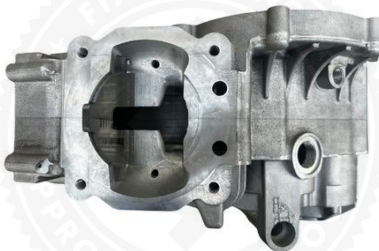
Photo du carter (côté joint) / Photo of the sump (gasket face)
